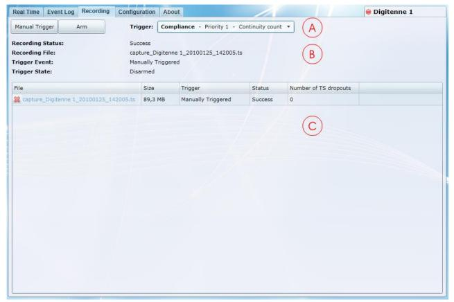
A: Trigger controls: used to define the trigger condition, arm the capture process or manually force a capture.
