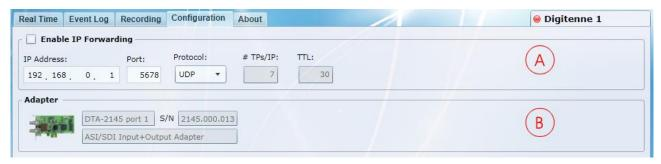
A: IP forwarding settings. Use to enable/disable forwarding of the monitored transport stream to a specific IP address.
