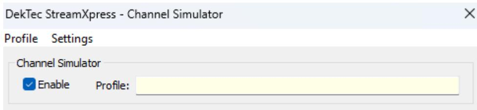
If checked, channel simulation is enabled, and noise and fading-path parameters can be specified. If unchecked, no channel simulation is applied.
