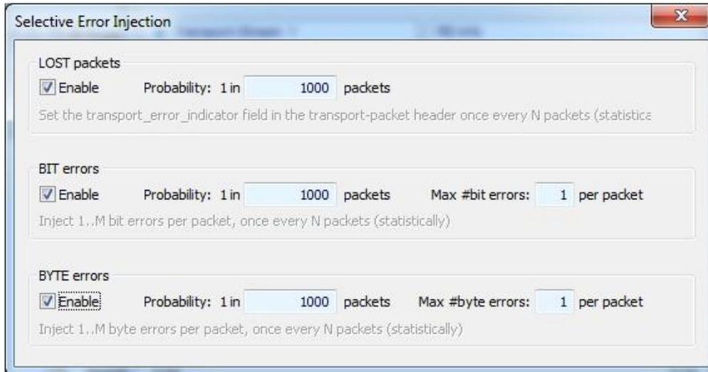
**Lost Packets:** When selecting this type of error insertion, StreamXpress will set the `transport_error_indicator` field in the TS packet header once every N packets. The frequency of the error insertion can be changed using the probability window.
