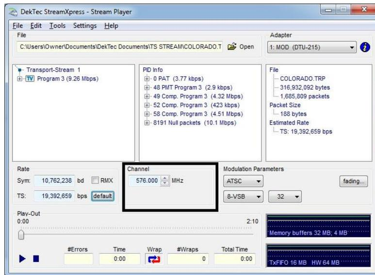
For example, if the modulated signal is 6 MHz wide and the selected RF channel frequency is 576MHz, the RF signal will span from 573MHz to 579MHz.
