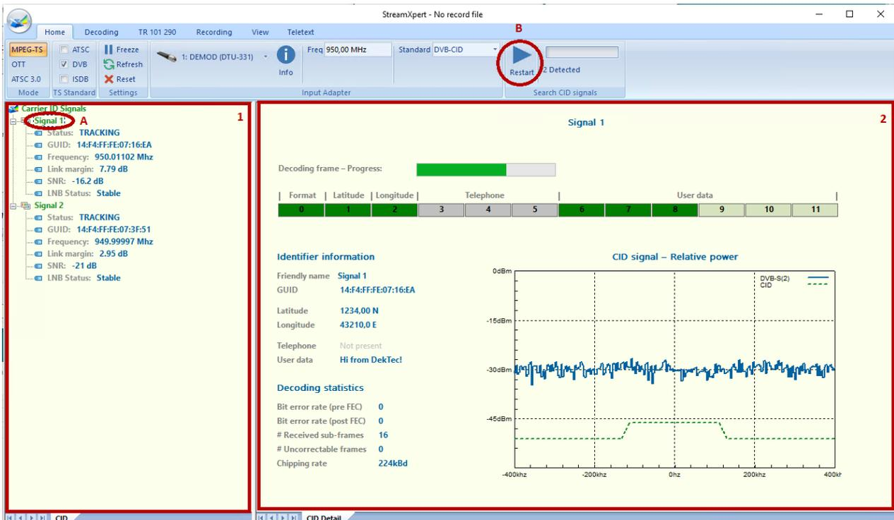
In the displayed graph, the real time spectrum is shown in blue, featuring both the DVB-S/S2 signal and DVB-CID signals. To provide an indication of the level of the DVB-CID signal in comparison to the DVB-S2 signal, the DVB-CID signal is represented by a dotted green line.
