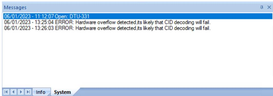
Figure 2. 'Messages' view in StreamXpert displaying hardware overflows
