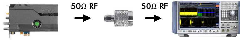
Figure 1. Hardware setup for measuring the performance of the DTA-2115B.
