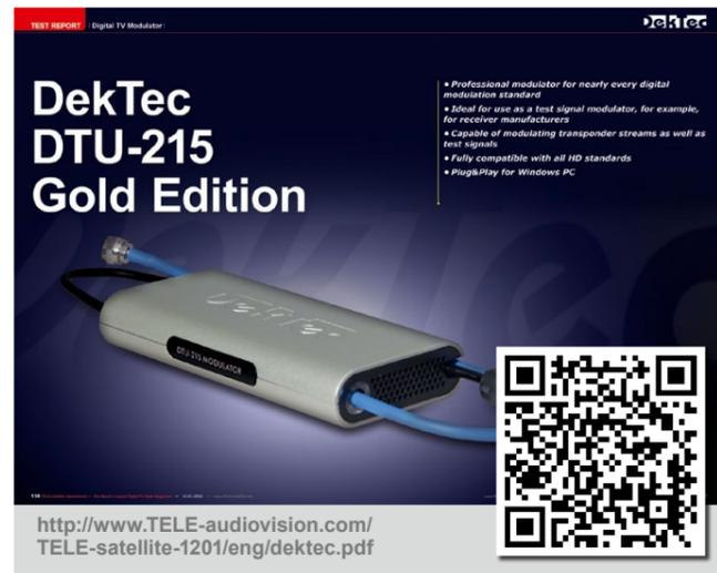
just needs a TS stream, preferably recorded in the region where the receiver will be used. This can then, with the DekTec modulator at a desired frequency and a desired modulation, be fed into a coax cable that is connected to the input of a receiver. And that's it. The manufacturer can now adjust at leisure the receiver's hardware and software until the signal is correctly demodulated.
